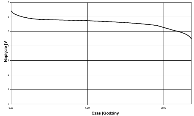
Run time for Maglite 3,5Ah rechargeable battery with 11W bulb
