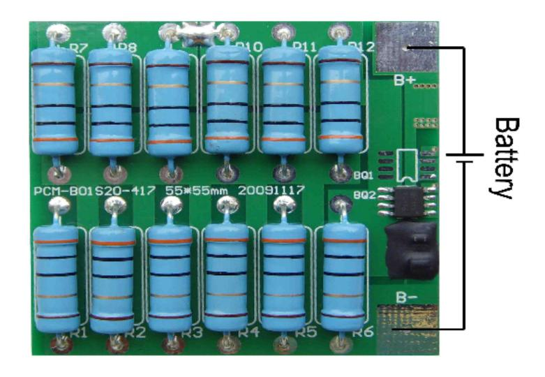
Remark: because of the high balancing current, it's better to take the wire abo∨e 18# for connection.
